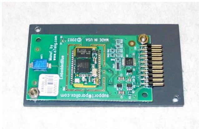
Figure#4. Embeddedblue transceiver mounted to deck.
