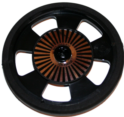
Figure#7. Attach WW-02 Encoder Disc to GM8 Wheel.
