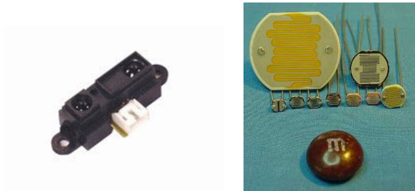
Figure 1. Sharp® GP2D120 Infrared Sensor and various cadmium sulfide photocells.
